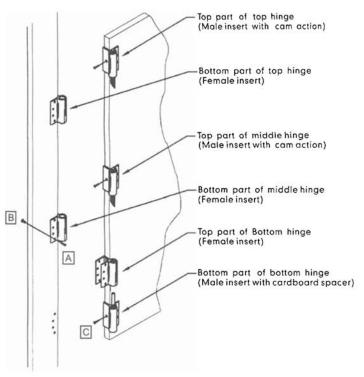
Note: Hinge barrel will be located on the same side that the door swings.
